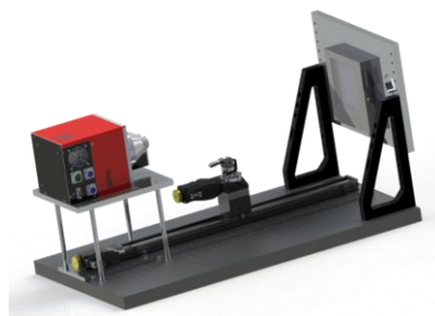
Fig 2. 3D rendering of X-ray μ-CT device at CelMat Laboratory
