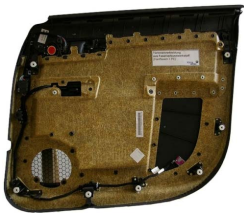
Figure I.1. Interior carpeting of a car door made on PE/hemp fibres biocomposite*.
