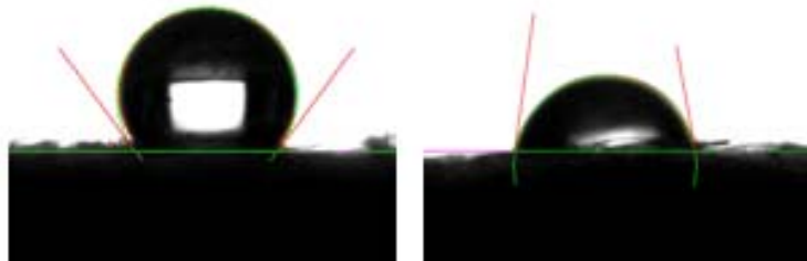
Figure II.22. Contact angle measurement.
