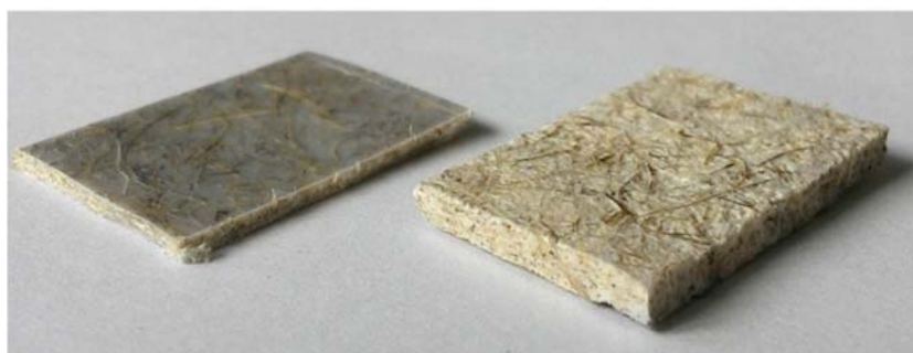
Figure VI.4. Comparative of the Untreated/PHB composites before and after expansion.
