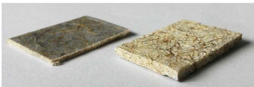
Composite material: before foaming (left) and after foaming (right).
