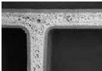
Figure 2.15: Detail of a structural foams. Two outer solid skins can be observed surrounding a foamed core.
