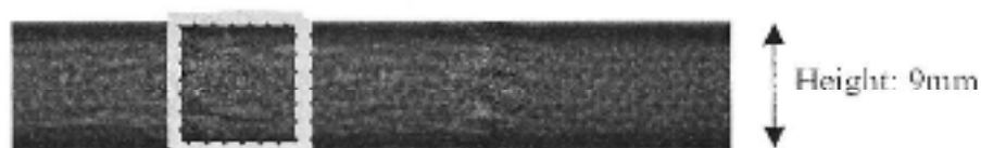
Figure 3. X-ray image of one typical structural foam. In grey is represented the analyzed area for vertical density profiles calculation
